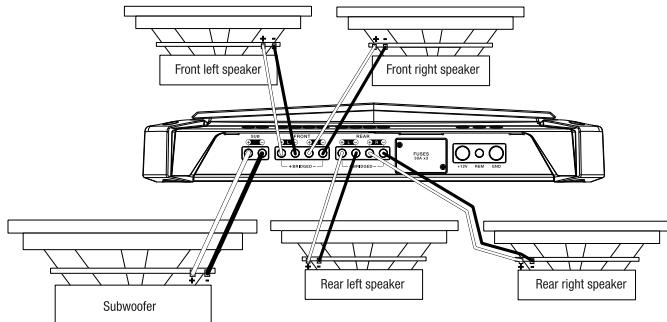
**OPMERKING:** Minimale luidsprekerimpedantie is 2 ohm.
