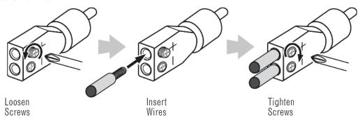
Always connect the (+) speaker wire to the adapter's (+) terminal and the (-) speaker wire to the adapter's (-) terminal. When all wires are connected, plug the adapters into the REF amplifier's FRONT (and REAR, if using the 4-channel amplifier) preamp inputs.
