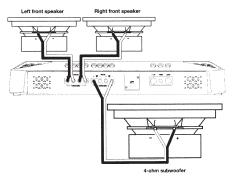
NOTE: You can connect two 2-ohm subwoofers in series to maintain the required 4-ohm mimimum impedance for the subwoofer channel.
