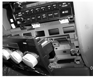
15. using your hand carefully unclip the right side of the climate controls from the radio and sub-dash and remove.
