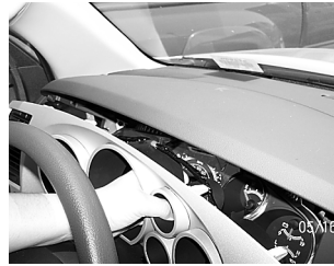
3. Using your hand pull from the center of the instrument cluster towards you.
