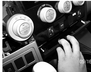
6. using your hand carefully pull and remove the bezel underneath the climate controls.
