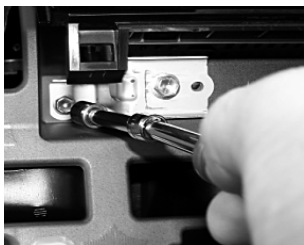
10. using a 10mm socket, remove the 2 10mm bolts holding the left side of the radio to the sub dash.
