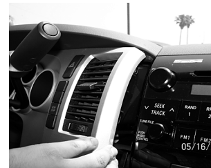
3. Using your hand, carefully pull the right side of the instrument cluster towards you.
