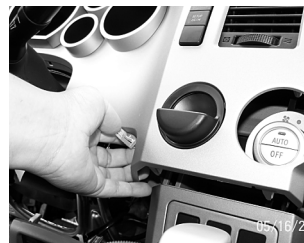
5. Using your hand, carefully pull the right side lower part of the instrument cluster towards you.
