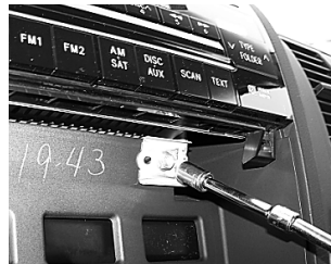
9. using a 10mm socket, remove the 2 10mm bolts holding the right side of the radio to the sub dash.
