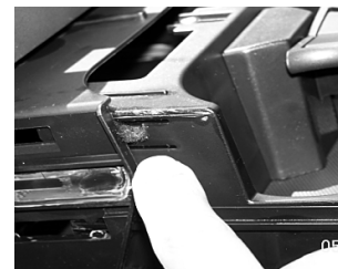
9. After stoppers have past the cup holder assembly, the cupholder is ready to slide out.
