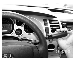
1. Lower column shifter all the way down and tilt the steering wheel all the way down.
