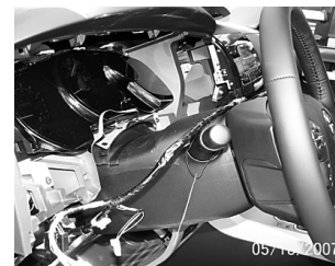
6. Disconnect harnesses and remove instrument cluster. Unclip sleeve from steering column.
