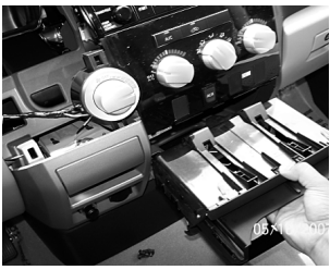
13. using your hand carefully pull the entire cup-holder cavity out.
