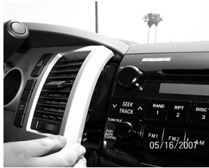
2. Using your hand, carefully pull the right side of the instrument cluster towards you.
