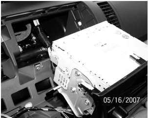
19. Pull radio completely out from the radio cavity and disconnect all harnesses.
