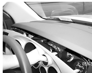
4. Using your hand pull from the center of the instrument cluster towards you.
