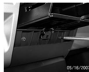
12. Remove 2 fillips head screws located underneath the cup holder cavity.
