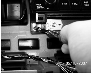
17. using a 10mm socket, remove the 2 10mm bolts holding the left side of the radio to the sub dash.
