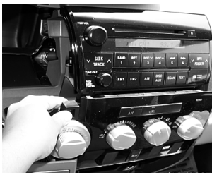
14. using your hand carefully unclip the left side of the climate controls from the radio and sub-dash.
