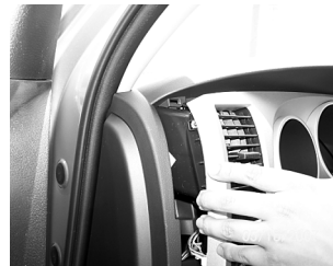
2. Using your hand, carefully pull the left side of the instrument cluster towards you.
