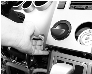
4. Using your hand, carefully pull the right side lower part of the instrument cluster towards you.
