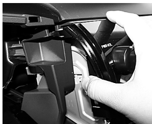
11. Carefully pull radio towards you and unclip from sub-dash.
