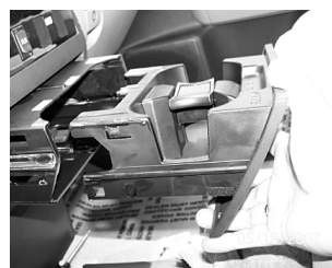
10. Slide the entire cup holder / tray completely out.
