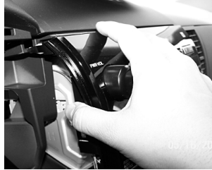
18. Carefully pull radio towards you and unclip from sub-dash.
