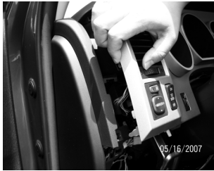
1. Using your hand, carefully pull the left side of the instrument cluster towards you.
