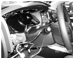
5. Disconnect harnesses and remove instrument cluster. Unclip sleeve from steering column.
