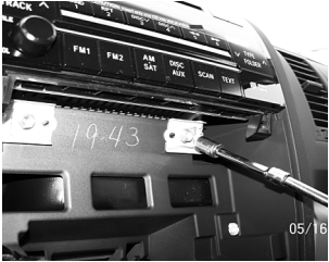
16. using a 10mm socket, remove the 2 10mm bolts holding the right side of the radio to the sub dash.
