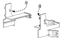
INSERT SPACER INTO BRACKETS ON BOTH SIDES ONLY WHEN ISO MOUNTING RADIO (ISO MOUNT HARDWARE INCLUDED)
